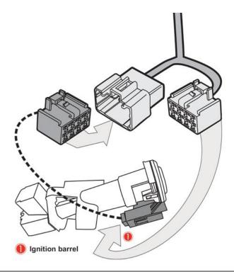
Secure the T harness so it does not cross any moving parts and reassemble the plastic cover.
