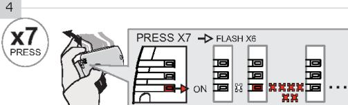
Press and release the programming button SEVEN (7x) times.
