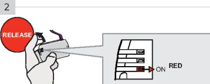
Release the programming button when the LED is RED.
